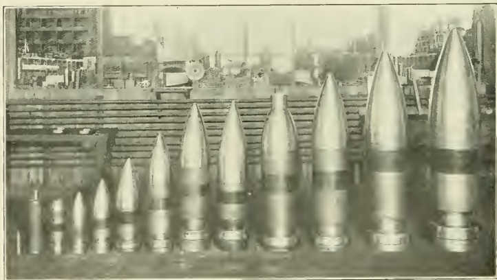
The picture shows projectiles which were made for guns of various calibers: 37 m. m. gun, 3.8 inch Howitzer, 4.7 inch Howitzer, 5 inch seacoast gun, 6 inch Howitzer, 6 inch seacoast gun, 8 inch Howitzer, 8 inch seacoast gun, 9.2 inch Howitzer, 10 inch seacoast gun, 240 m. m. Howitzer, 12 inch seacoast gun, 12 inch seacoast mortar, 14 inch gun, and 16 inch gun. These shells were made by the Superior Machine Tool Company, Kokomo, Ind.
